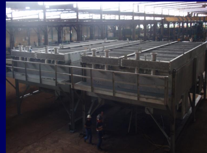
“U” Tubes, 2964 Tubesheet Holes. Tubes Inconel 625 (SB 444-1) & Tubesheets SA336 – 304 Forges SA336 F11-CL3
