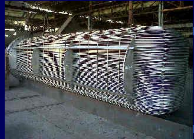
“U” Tubes, 2964 Tubesheet Holes. Tubes Inconel 625 (SB 444-1) & Tubesheets SA336 – 304 Forges SA336 F11-CL3
