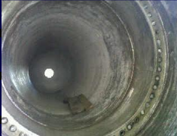
“U” Tubes, 2964 Tubesheet Holes. Tubes Inconel 625 (SB 444-1) & Tubesheets SA336 – 304 Forges SA336 F11-CL3
