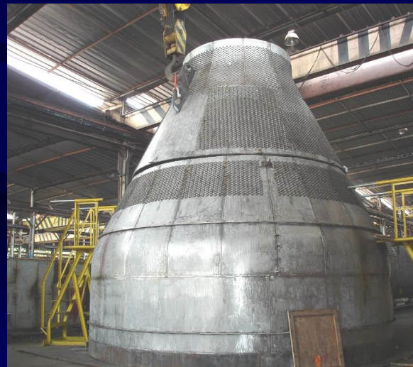
Riser Cone Diam 7.2 m, SA347 H S.S
