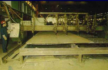
Multi Torch Flame Cutting
