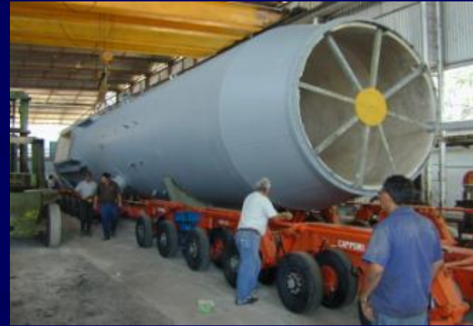
Stack 140 Mtons , with Refractory
