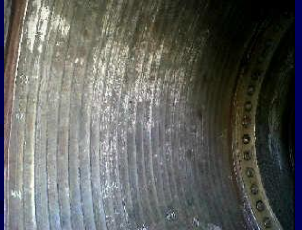
“U” Tubes, 2964 Tubesheet Holes. Tubes Inconel 625 (SB 444-1) & Tubesheets SA336 – 304 Forges SA336 F11-CL3
