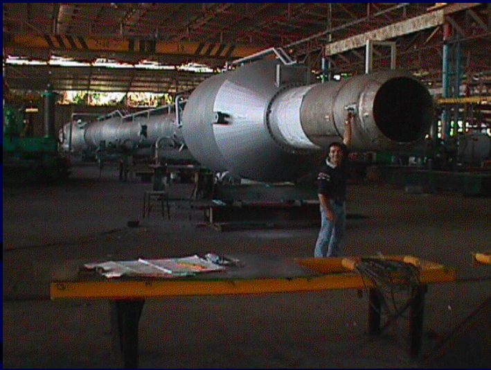
Equipments delivered with Castables poured at shop floor
