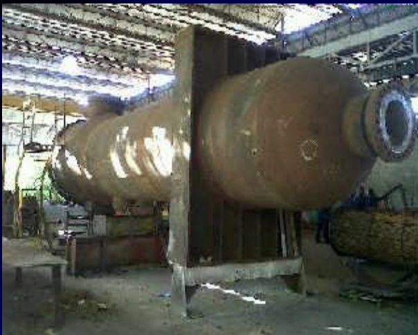
“U” Tubes, 2964 Tubesheet Holes. Tubes Inconel 625 (SB 444-1) & Tubesheets SA336 – 304 Forges SA336 F11-CL3
